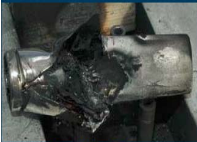
Fire with Case Rupture
