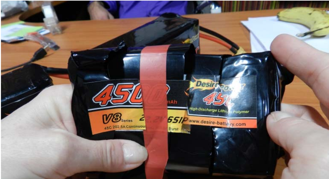
Picture 1. Outside label and cover removed from a 12,400 mAh lithium battery
