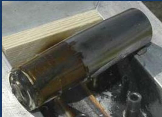
Fire with Cell Venting
