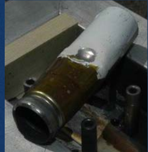
Fire with Energetic Disassembly
