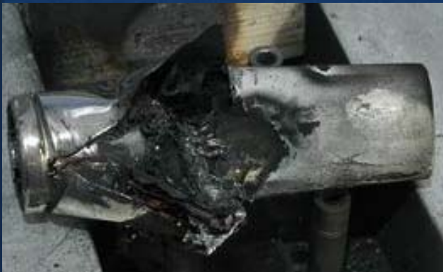
Fire with Case Rupture
