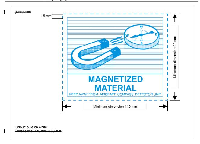
Figure 5-2425. Magnetized material
