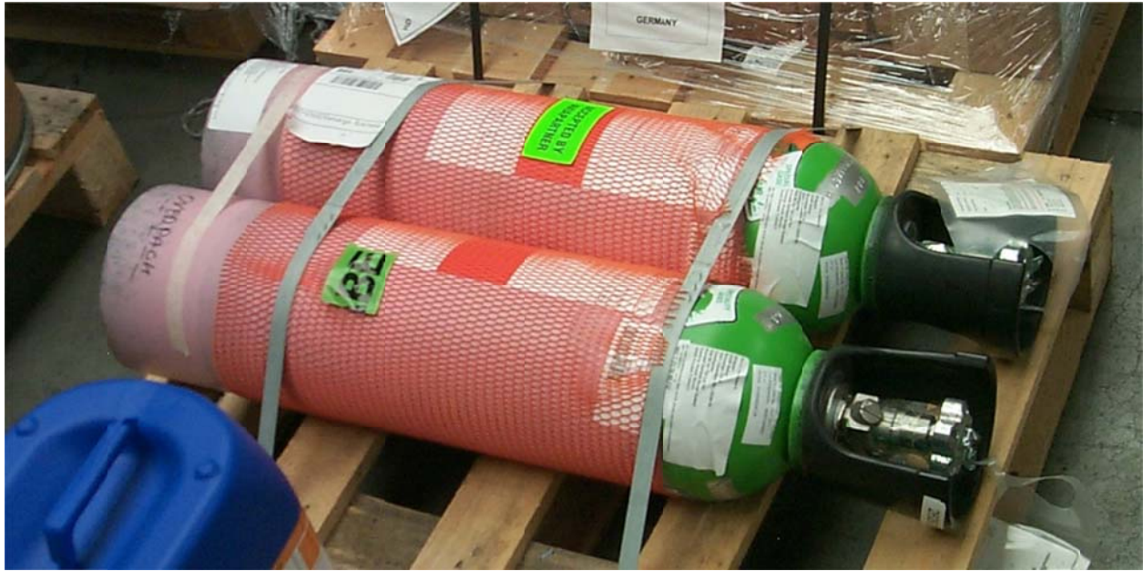
Figure 1 - Two cylinders fastened to a pallet but not interconnected by a manifold
