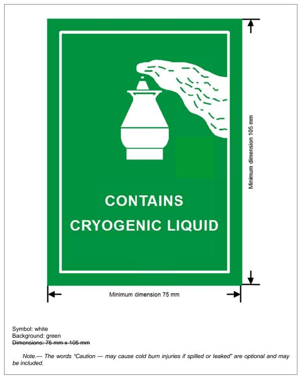
Figure 5-28. Cryogenic liquid label
