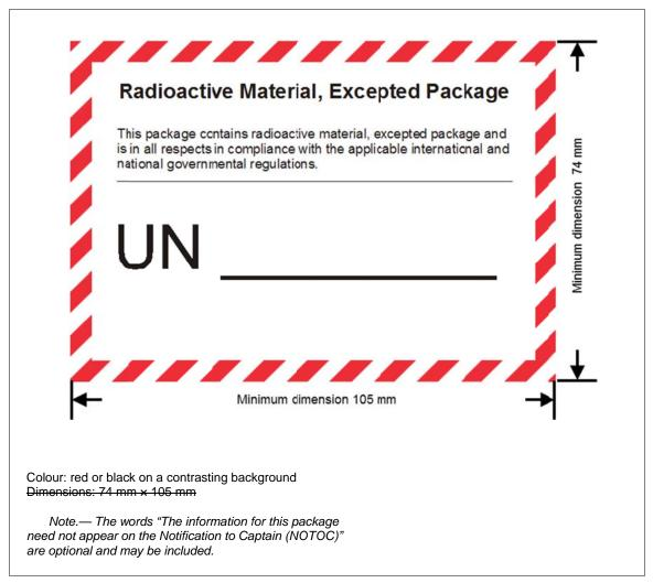
Figure 5-30. Radioactive material, excepted package
