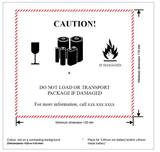
Figure 5-31. Lithium battery handling label
