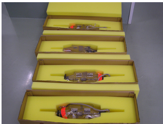
(Inside of Inner Package--- After the Test) 内装梱包状態 落下試験後
