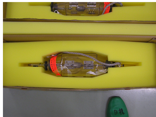
(Inside of Inner Package---After the Test (2)) 内装梱包状態 落下試験後(2)
