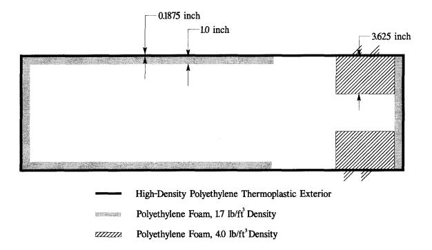
FIGURE 5. SCHEMATIC OF STANDARD VIKING OVERPACK CONSTRUCTION
