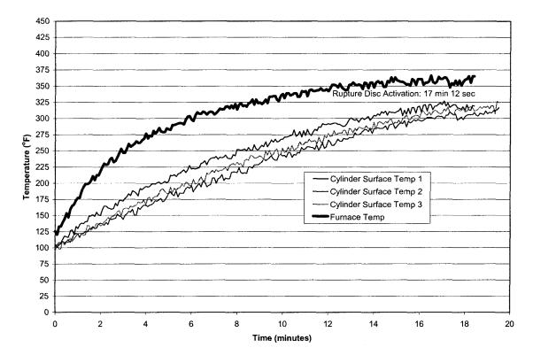
FIGURE 4. FURNACE TEST RESULTS USING 11-CUBIC-FOOT CYLINDER
