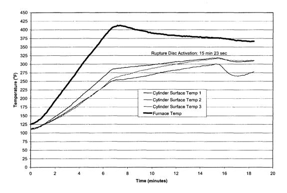
FIGURE 3. FURNACE TEST RESULTS USING 115-CUBIC-FOOT CYLINDER
