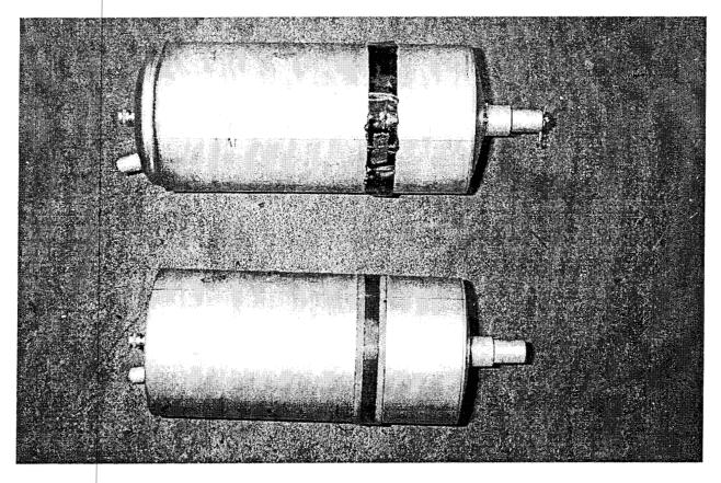
FIGURE 2. OUTWARDLY BULGED GENERATOR AND NORMAL GENERATOR
