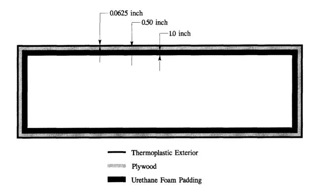
FIGURE 9. SCHEMATIC OF ANVIL OVERPACK CONSTRUCTION
