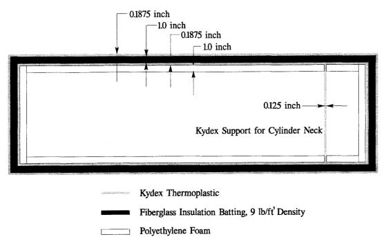
FIGURE 11. MODIFIED VIKING OVERPACK USING FIBERGLASS BATT INSULATION
