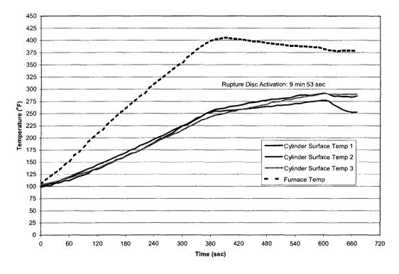
FIGURE 2. FURNACE TEST RESULTS USING 76.5-CUBIC-FOOT CYLINDER
