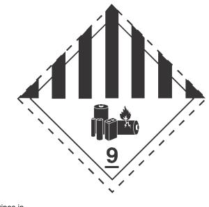
Symbol (seven vertical stripes in upper half); battery group, one broken and emitting flame in lower half: black Background: white Figure "9" underlined in bottom corner
