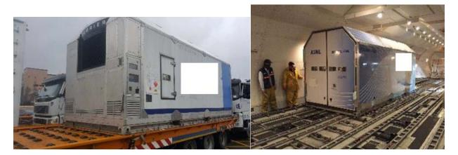
1.5 To facilitate the acceptance and carriage of this type of machinery it is proposed to include into Packing Instructions 378 and 972 the provisions for vehicles from Packing Instruction 950. For Packing Instruction 972 it is questioned as to whether there is any need to drain the fuel tank as the fuel must be non-flammable.
