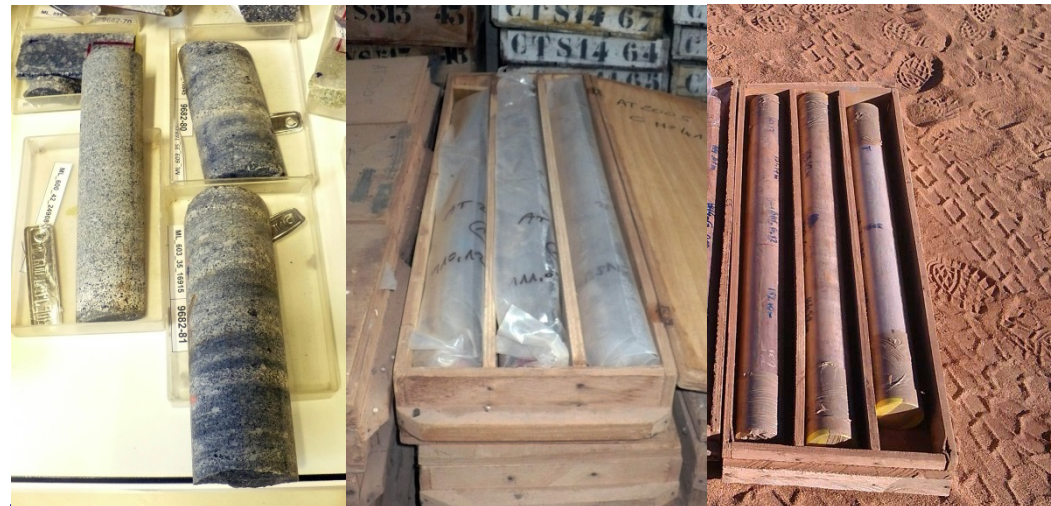
Geologic carrots (rocks, 8 cm in diameter, up to 1 m long, up to 15 kg each) in plastic tubes closed by adhesive tape, or in plastic sleeves, placed in a rack, made of plywood or natural wood
