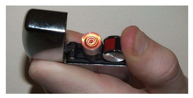
Figure 1 -Flameless electronic lighter with the heating coil activated. \\
