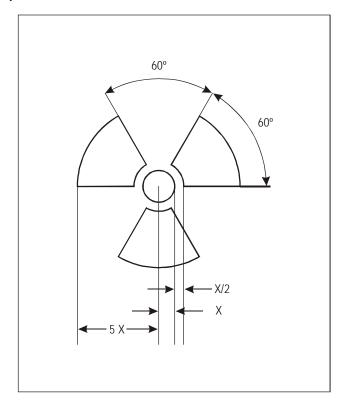
Figure 5-1. Basic trefoil symbol with proportions based on a central circle of radius X. The minimum allowable size of X must be 4 mm.
