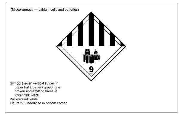
Figure 5-25. Miscellaneous dangerous goods — lithium batteries, Class 9
