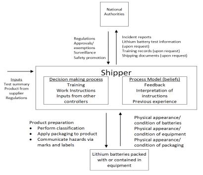
Figure 2. Control-feedback loop for a shipper
