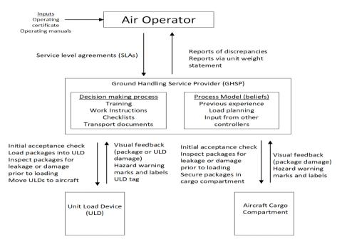
Figure 3. Control feedback loop for a ground handling service provider
