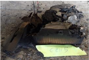
Battery package and casing burned/melted Cell shrink-wrap (label) melted
