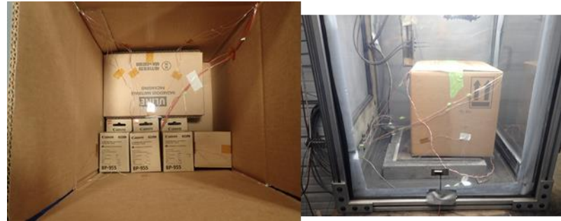
3x3 batteries with trigger battery in the center
