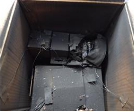
Flap opened during test Multiple cells with contents ejected
