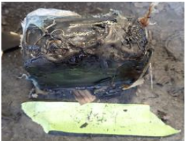
Battery package and casing burned/melted Cell shrink-wrap (label) melted
