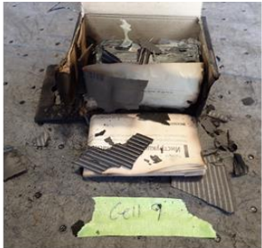
Flap opened during test Multiple cells with contents ejected
