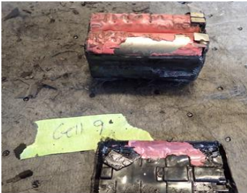
Flap opened during test Multiple cells with contents ejected
