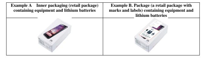
1.2.1 **Scenario 1.** If four of the boxes shown in Example A are put into an outer packaging, the requirements of Packing Instruction 966, Section II would apply and the package would be subject to the 1.2 m drop test requirement.
