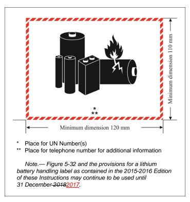
Figure 5-3. Lithium battery mark
