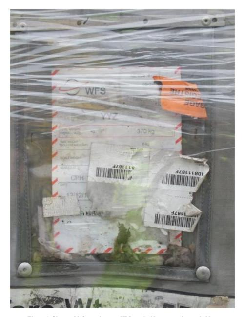
Figure 1. Obscured information on a ULD tag inside a protective tag holder
