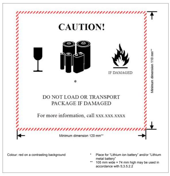
Figure 5-32. Lithium battery handling label
