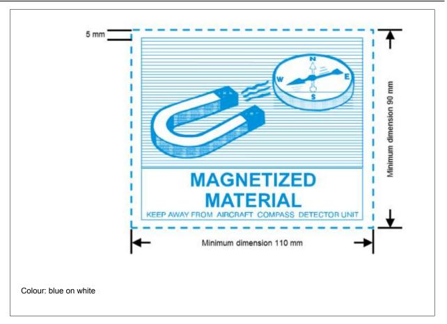
Figure 5-25. Magnetized material
