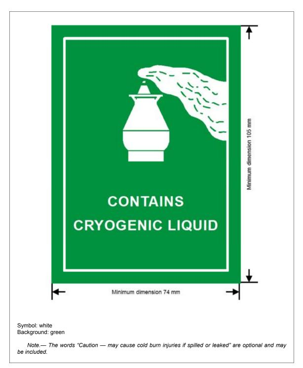
Figure 5-29. Cryogenic liquid label
