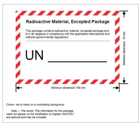
Figure 5-31. Radioactive material, excepted package
