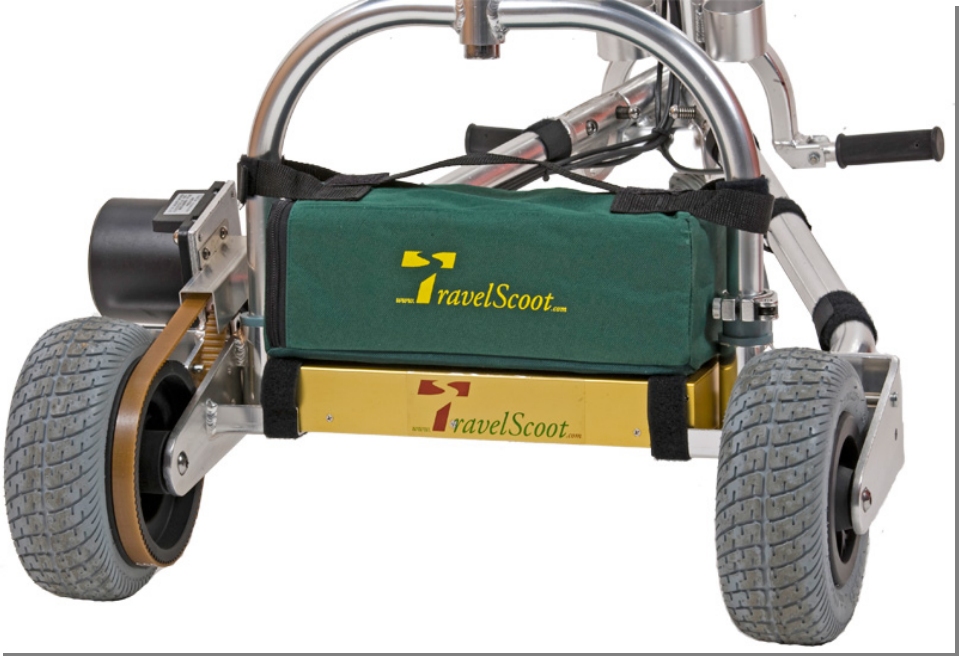
Figure 2. Rear view of battery (gold metal rectangular item), green pack is a second battery that “can” be added.
