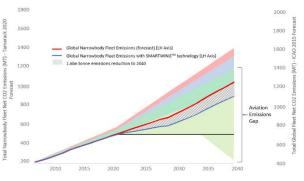
SMARTWING technology application on Global Narrowbody Fleet could close ICAO CO<sub>2</sub> Emissions Gap by 1.6bn Tonnes (20%) by 2040
