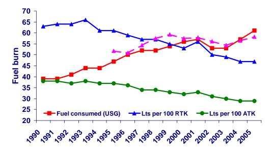
**Figure 1 - Fuel consumption vs capacity evolution**AAGR – Average Annual Growth Rate; ATK - Average tonnes km; RTK – Revenue tonnes km
