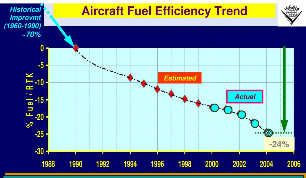
~ 70% Fuel Efficiency improvement up to 1990 at product level Continuing improvement reflected at fleet level (average > 1.5%/year) Driven by strong & efficient market forces, combined with inherent fastevolving high technology & improved operational practices Needs sustained research & technology funding from Industry & Governments
