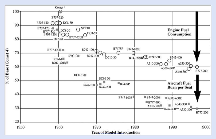
\_IPCC Special Report on Aviation And the Global Atmosphere **Figure 9-3:** Trend in transport aircraft fuel efficiency.
