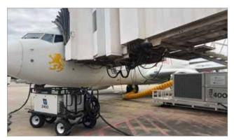
Gate equipment (GPU and PCA) funded by the project is connected for the first time to an international flight at Moi International Airport, Mombasa, Kenya
