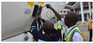
Gate equipment (GPU) is being connected to power aircraft during ground operations which avoids the use of jet-fuel powered APUs
