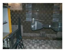
Model Rotor Testing at DNW
