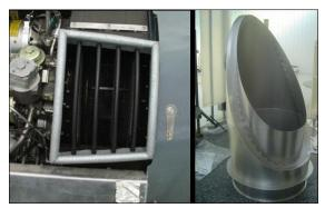
*Figures:* Acoustically treated additional lateral air inlet to the compressor chamber (left) and treated ejector (right)
