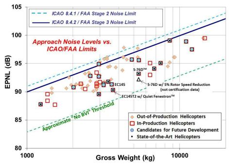
Figure 7. Chapter 8 Approach Noise Levels vs. Gross Weight Showing Current Best-in-Fleet Margin to 8.4.1 and 8.4.2 Limits, Example Case of N<sub>R</sub> Reduction, and Approximate "No BVI" Margin Threshold
