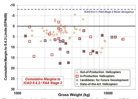
**Figure 1. Cumulative Margins to 8.4.2 Noise Limits for Chapter 8 Helicopters** (Note that the ordinate values on this plot have been reversed for presentation purposes.)
