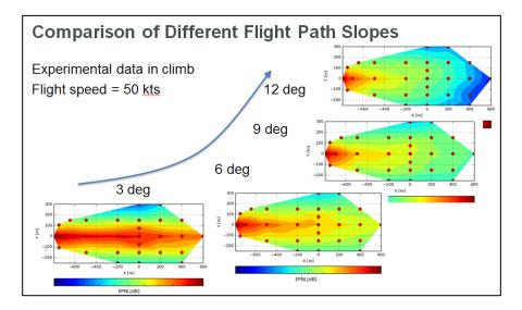
Figure: Comparison of Helicopter acoustic footprint at different climb slopes as measured in CleanSky
