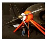
*Figure:* active flap rotor in S1-Modane wind tunnel
