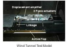
maximum cruising speed of a helicopter in order to demonstrate the proper operability of the active flap system on more realistic environment.
