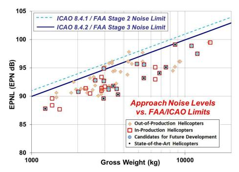
Figure A-2. Chapter 8 Approach Certification Noise Levels vs. 8.4.1 and 8.4.2 Noise Limits
