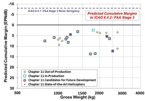
Figure 2. Predicted Cumulative Margins to 8.4.2 Noise Limits for Chapter 11 Helicopters (Note that the ordinate values on this plot have been reversed for presentation purposes.)
