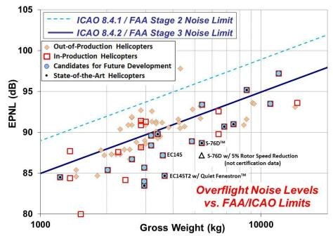
Figure 8. Chapter 8 Overflight Noise Levels vs. Gross Weight Showing Current Best-in-Fleet Margin to 8.4.1 and 8.4.2 Limits and Example Case of N<sub>R</sub> Reduction
