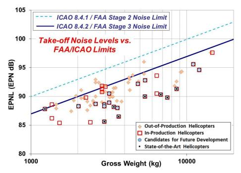
Figure A-1. Chapter 8 Take-off Certification Noise Levels vs. 8.4.1 and 8.4.2 Noise Limits
