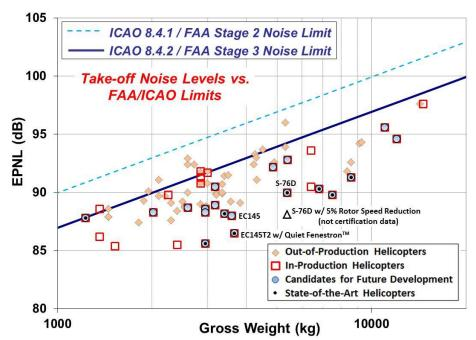
Figure 6. Chapter 8 Take-off Noise Levels vs. Gross Weight Showing Current Best-in-Fleet Margin to 8.4.1 and 8.4.2 Limits and Example Case of N<sub>R</sub> Reduction
