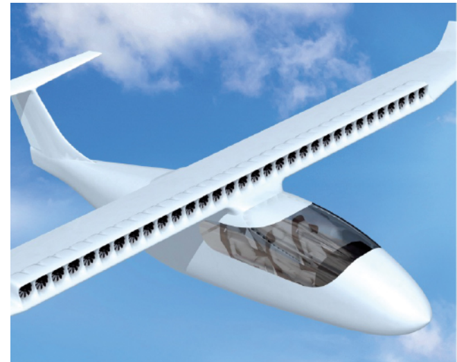
Ampere Project: ONERA concept of distributed electric propulsion aircraft
