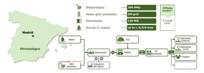
FIGURE 1: Scheme of the Montealegre project
