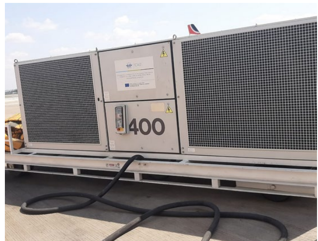
FIGURE 8: Pre-conditioned air (PCA)
