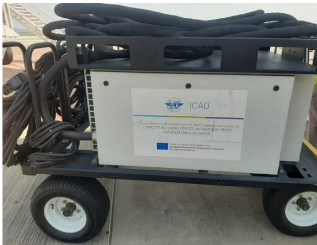
FIGURE 7: Ground power unit (GPU)
