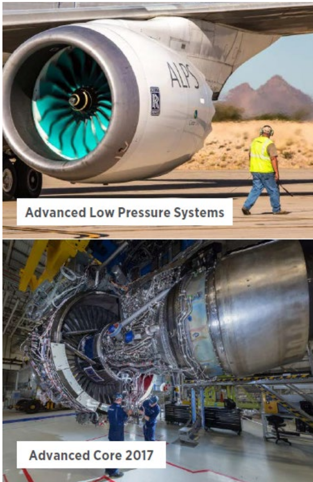
FIGURE 6: a. & b. Clean Sky 2 Demonstration engines showing advanced Low Pressure (LP) and High Pressure / core technology
