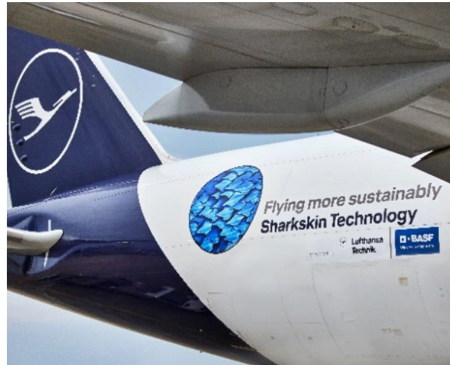
FIGURE 3: Airline based testing of skin riblet drag reduction (Deutsche Lufthansa, Oliver Roesler)
