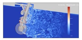
• <u>Semi-empirical methods</u>: The phased-array and computational aeroacoustic results were used to enhance traditional semi-empirical methods for the prediction of airframe noise.
