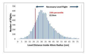
to estimate lateral efficiency—the 15<sup>th</sup> percentile of actual distance flown in level flight within 40nm of destination (see Figure 7).
