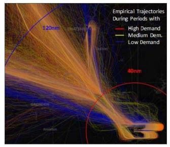
FIGURE 11: Variance in Vertical Profiles of Empirical Trajectories for Flights Arriving to ATL via NW Corner Post during West Airport Flow and for Different Demand Levels in 2016
