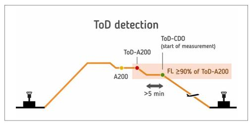
In 2015, EUROCONTROL set up the European CCO-CDO Task Force to solve this issue and developed a set of harmonized CCO-CDO definitions, metrics, and parameters for measuring CCO-CDO, as agreed by stakeholders. These include harmonized definitions of both a fuel CCO-CDO (to top of climb or from top of descent, respectively), and a noise CCO-CDO (from FL75 or to FL105, respectively) lower levels where noise is the primary environmental impact.
