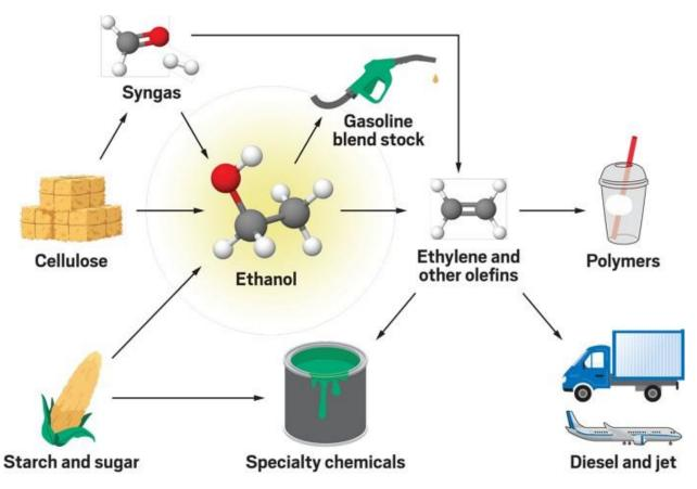
Figure 802. Ethanol as an intermediate to make fuels and chemicals from biomass
