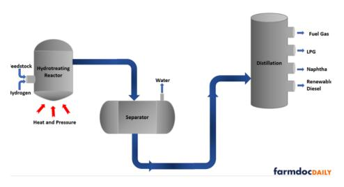
Figure 257. HVO renewable diesel production process
