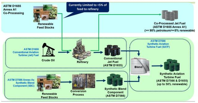
Figure 280. SAF co-processing process
