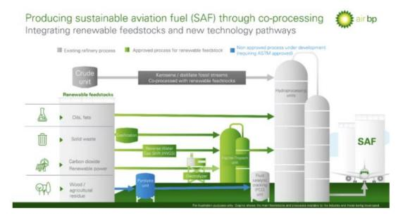
Figure 29. Co-processing pathways using various renewable feedstocks.
