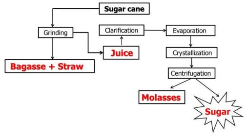
Figure 335. Sugarcane Processing By-products
