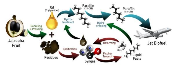
Figure 724. Process to Produce SAF From Jatropha Fruit
