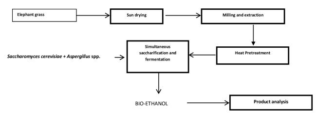
Figure 58. Process to make bioethanol from elephant grass
