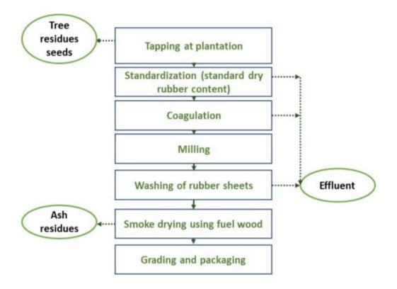
Figure 613. Rubber production process
