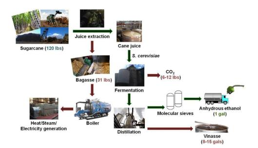
Figure 368. Biofuel production process from sugarcane juice
