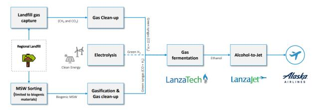
Figure 824. ATJ SAF Process From MSW Feedstock
