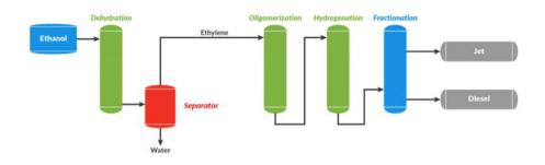
Figure 20. ATJ SAF conversion process from ethanol
