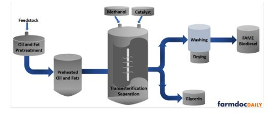
Figure 246. FAME biodiesel production process
