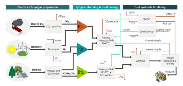
Figure 235. PtL SAF conversion process from carbon dioxide and biomass
