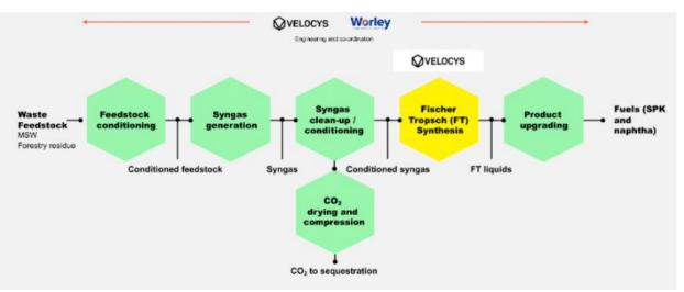
Figure 835. FT SAF process from MSW and forestry waste
