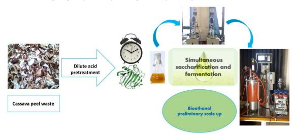
Figure 424. Process to produce bioethanol from cassava peels
