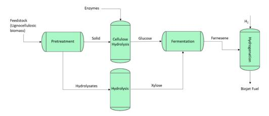
Figure 21. SIP-HFS/DSHC SAF Conversion Process from Biomass
