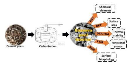
Figure 413. Biochar Production from Cassava Peels
