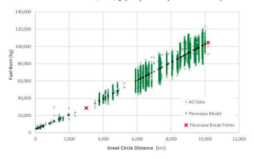
Figure 8: Illustration of fuel burn statistical method model formulation (GCD Model)
