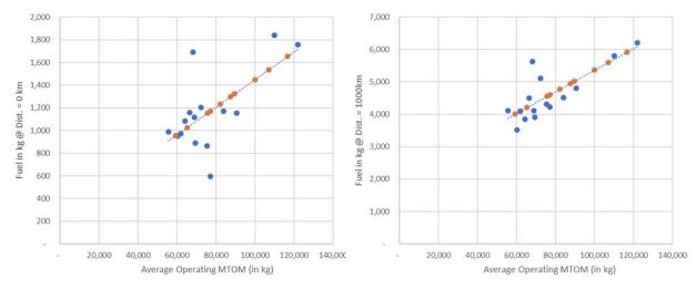
Figure 10: Illustration of generic aircraft fuel burn-MTOM based regressions for a given distance
