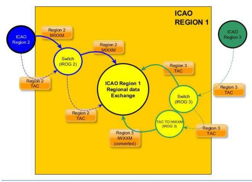
Figure 6: Phase 2, interregional exchange of OPMET with Region 2 (IWXXM & TAC capable) and Region 3 (TAC capable)
