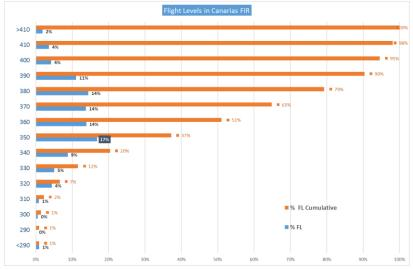
Figure 2. Distribution the Flight Levels in EUR/SAM Corridor – Canarias FIR
