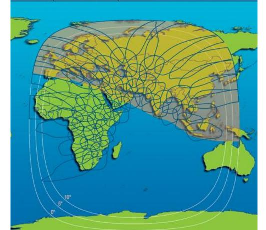
Ku-band Multi-Spot & Wide Beams Peak up to 61.6 dBW
