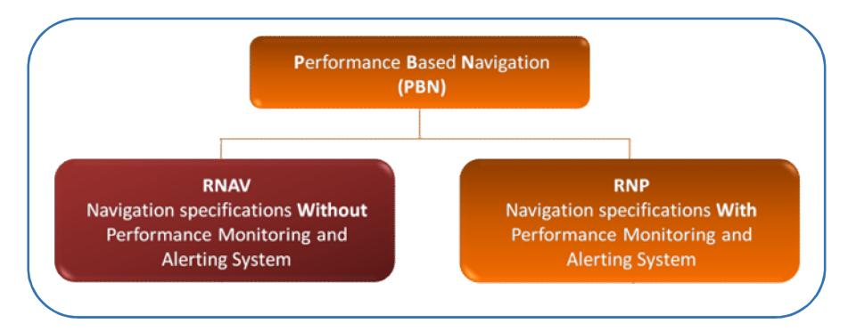
**RNP = RNAV + OPMA** (On-board Performance Monitoring and Alerting)
