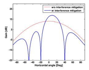
FIGURE D6  $\label{eq:matterns} \textbf{IMT-Advanced base station radiation patterns (Nt = 8, Nes = 6) }$
