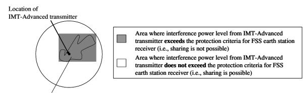
Interference power level is non-uniformly decreased due to shielding effect
