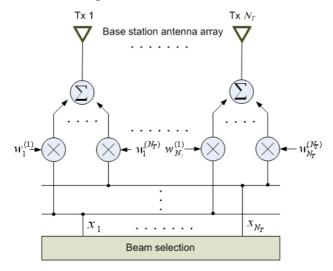
A linear array of  $N_T$  isotropic antenna elements with uniform spacing is considered. The data signals  $x_k$ ,  $k = 1, \dots, N_T$  from the beam selector are direct multiplied by a set of weights  $U = \{\mathbf{w}_1, \mathbf{w}_2, \dots, \mathbf{w}_{N_T}\}$  to form a null at known DOE.  $\mathbf{w}_m = [w_1^{(m)}, w_2^{(m)}, \dots, w_{N_T}^{(m)}]$  is the m-th weight vector in row vector and is given by the following set of equations:
