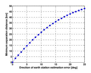
TABLE D1  $\label{eq:table_def} \mbox{Minimum required separation distance for different (Nt = 4, Nes = 1) }$
