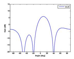
FIGURE D5 IMT-Advanced base station radiation patterns (Nt = 4, Nes = 3)
