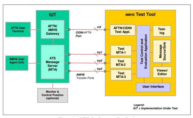
Figure 1: AMHS Conformance Test Environment
