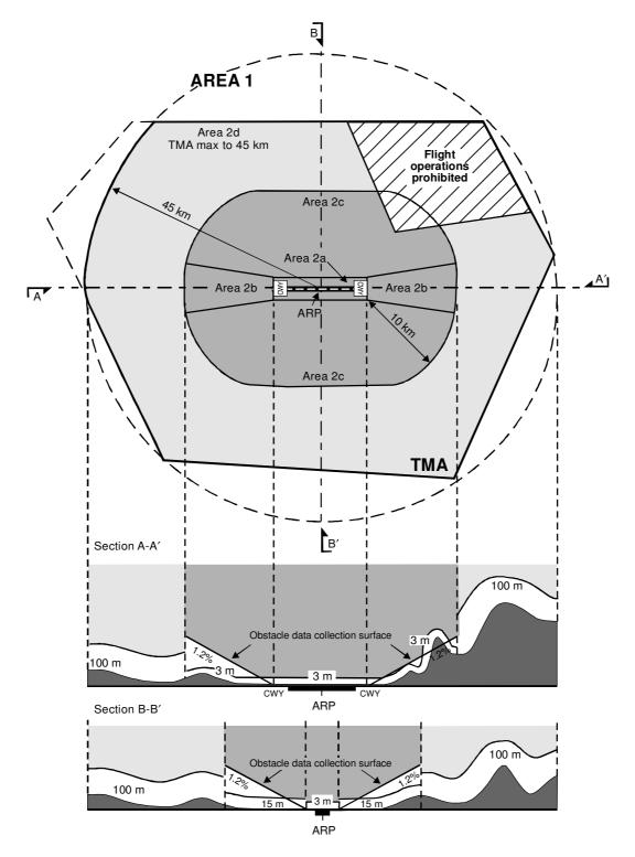
**Figure A8-2.** Obstacle data collection surfaces — Area 1 and Area 2 Edit Note: Figure A8-2 needs to be revised to reflect the changes to Area 2b but we do not have the source available to make the necessary changes.
