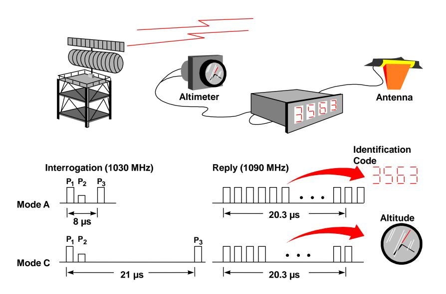
Synchronous Garbling of Transponder Replies (A problem in busy areas resulting in some aircraft not being detected)
