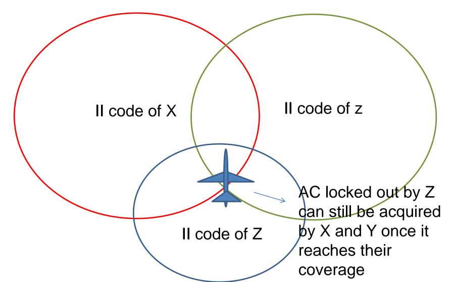
Examples of how limited II codes (0 to 15) should be used judiciously! For a handful of radars, manual assignment of codes is
