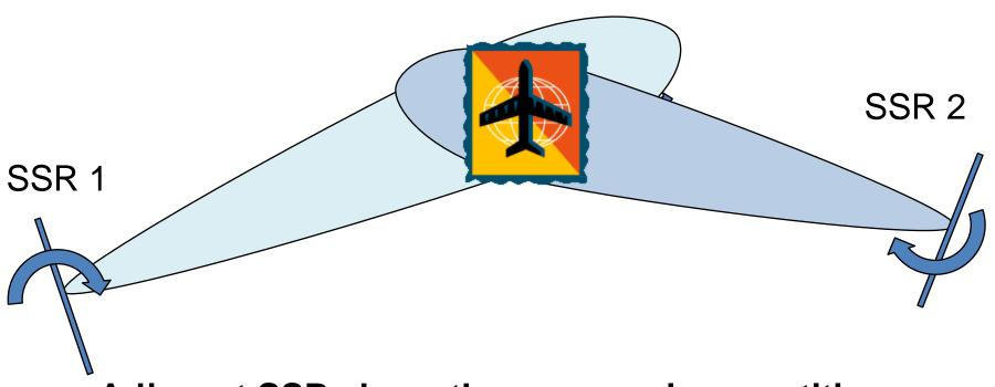
Adjacent SSRs have the same pulse repetition frequencies (PRFs) – if pulses collide or are too close, the aircraft won't be detected
