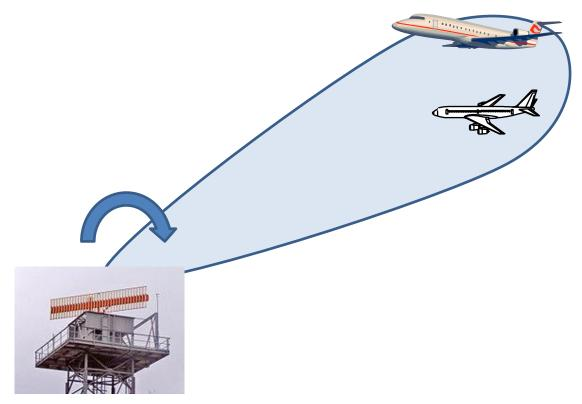
However, Mode S can do adoptive interrogations. The Stochastic All-call interrogation asks for replies to be sent with a probability of less than 1. Chances are the two A/Cs come up with different probabilities so both don't reply to each interrogation. So both are acquired.
