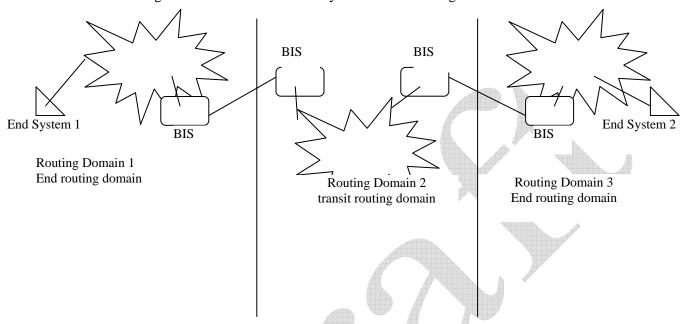
Note: A transit routing domain may or may not be part of the backbone. That is, a routing domain may consist of BISs none of which are backbone routers.
