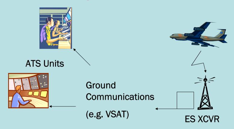
A proper ground infrastructure is required to ensure timely delivery of ADS-B messages to ATS units. The system should provide proper availability, integrity, transit time and so on in order for the data to be operationally useful.
