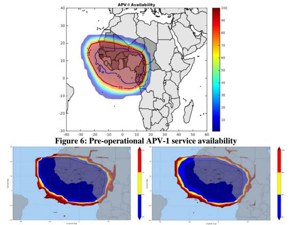
Figure 7: Pre-operational OS service availability (left: horizontal accuracy 3m@100%, right: vertical accuracy 4m@100%)
