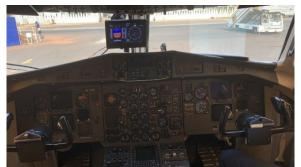
Figure 9: Flight deck equipped with navigation display for SBAS demo flight
