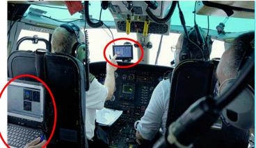
Figure 12: Flight deck with external navigation display for SBAS demo flight
