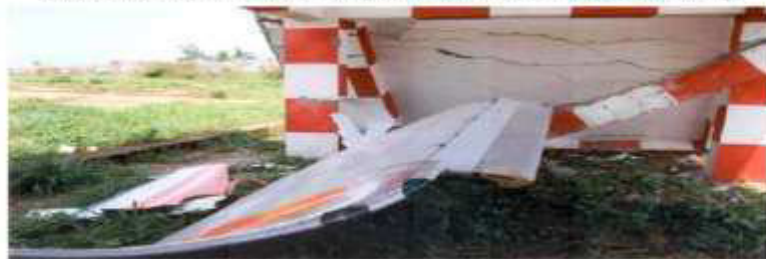
Photo 10: Broken Wing of Aircraft after Impacting the ILS Mounting Structure
