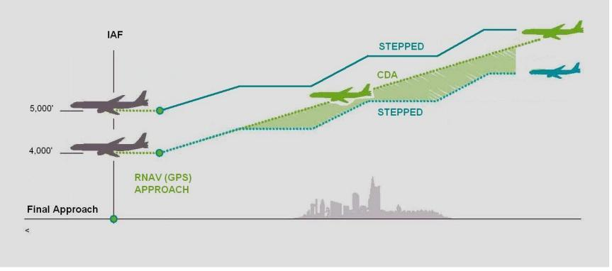
STAR altitude windows and procedure height constraints should be designed to allow most aircraft to descend unimpeded.
