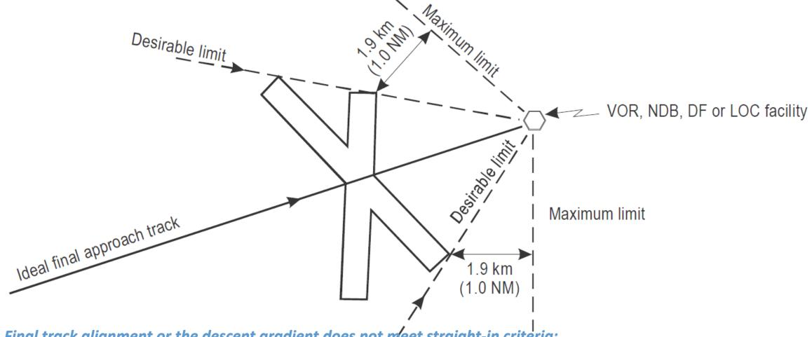
Final track alignment or the descent gradient does not meet straight-in criteria:
