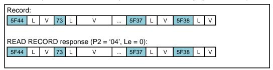
Case b — Read several records up to the file end (the Le field contains only bytes set to '00')
