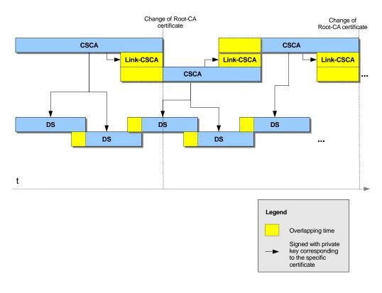
Figure 1: Re-keying process of CSCA certificates
